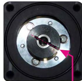
The inner and outer slit is aligned as they should.
