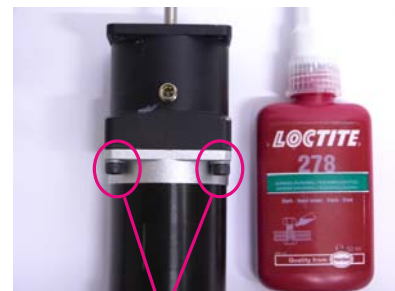
Flange bolts properly mounted and tightend.
