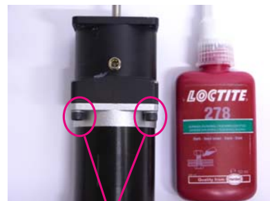
Flange bolts properly mounted and tightend.
