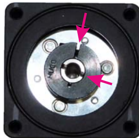
The inner and outer slit is NOT aligned. Make sure they are aligned as shown at right illustration
