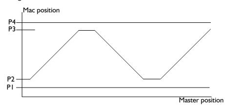
As illustrated, the stop positions are given by the values of registers P2 and P3.
