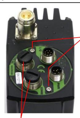
Use protective caps on unused connectors. Tighten properly.
