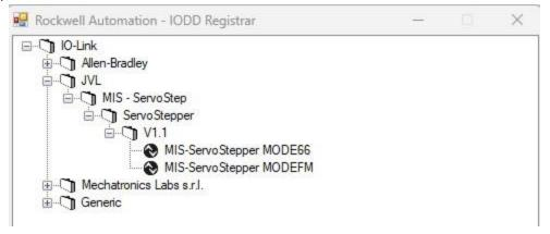
2. For the relevant channel, select which JVL device is connected. Note that by default, Mode66 is activated.
