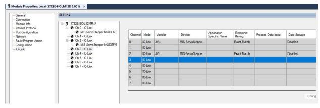
3. Download the configuration to the PLC and make sure the motor is connected to the IO-Link master and power supply.
