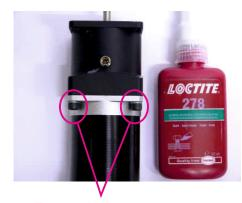
Flange bolts properly mounted and tightend.
