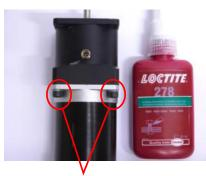
Properly mounted and tightened flange bolts.
