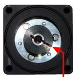
Correctly aligned inner and outer slits.
