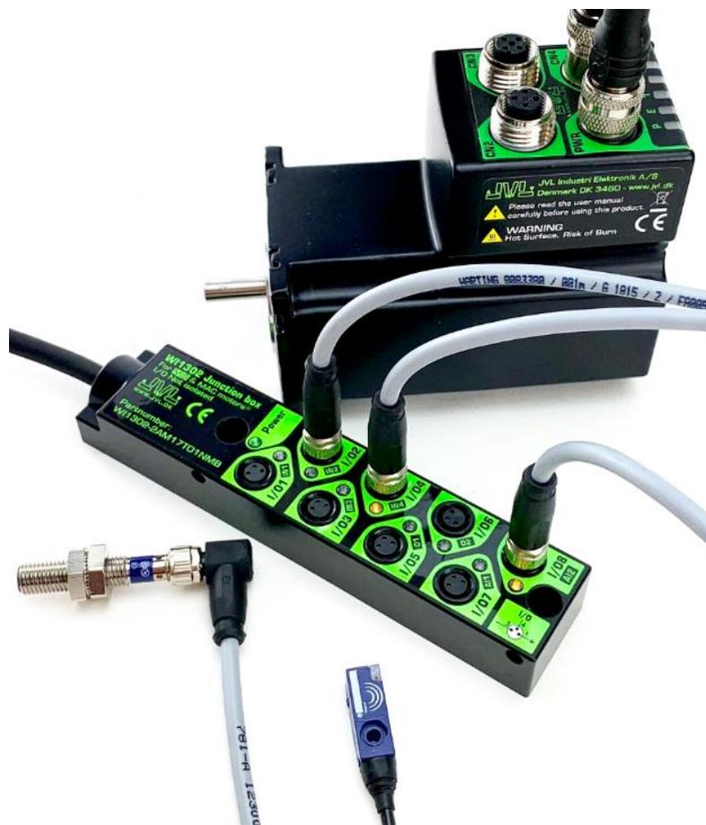
**Plug-and-play Junction Box for standard M8-3pin sensors and devices. Just connect the Junction Box to your integrated servo or stepper motor and up to 8 local 24 VDC I/Os are available.**
