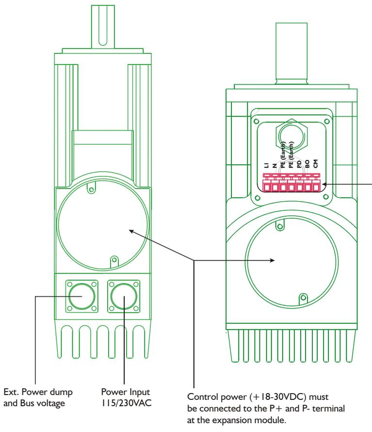
Main power, internal bus voltage and power dump is accessible through these spring contacts placed under the top lid. Main power must be 115 or 230VAC.
