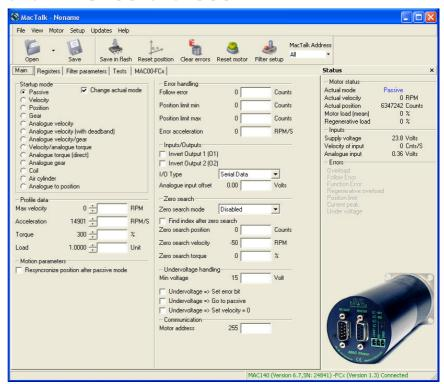
With JVL's MacTalk software it is easy to setup and diagnose a MACxxx integrated servo motor.
