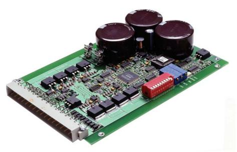
This driver is an advanced multi-function step motor driver which can be controlled both by external step pulses, but also from an internal step generator which controls the speed, acceleration etc. of the motor.
