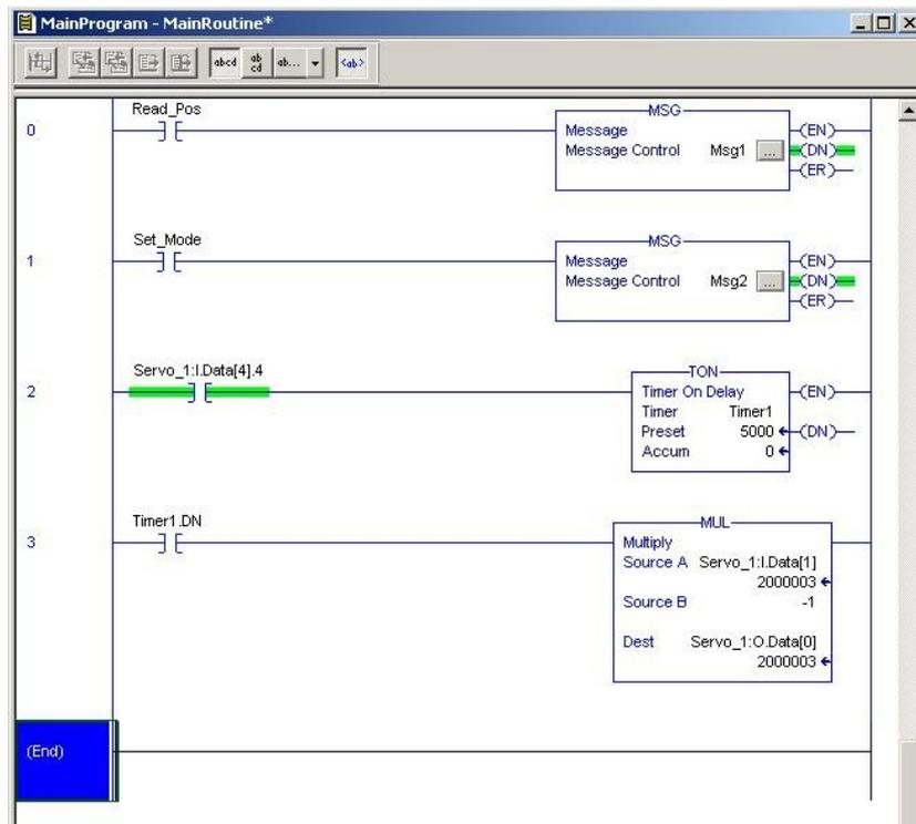
Rung nr. 1 will take care of sending an explicit message, that copies the value from the "Mode"-tag into the mode register in the motor as soon as the boolean "Set\_Mode" -tag is set. This example is based on the motor being put into "Position" -mode.
