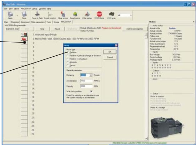
**6** Choose the movement type needed. Relative: Move x counts forward with reference to the actual position. Absolute: Move to the x position with reference to the zero search position.
