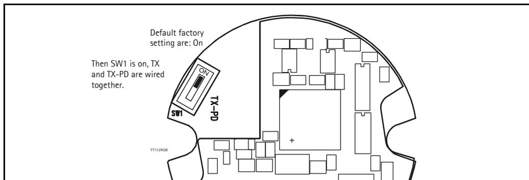
If the MAC motor is connected to the same RS232 line as other motors, the terminal TX-PD should only be connected on one of the motors.
