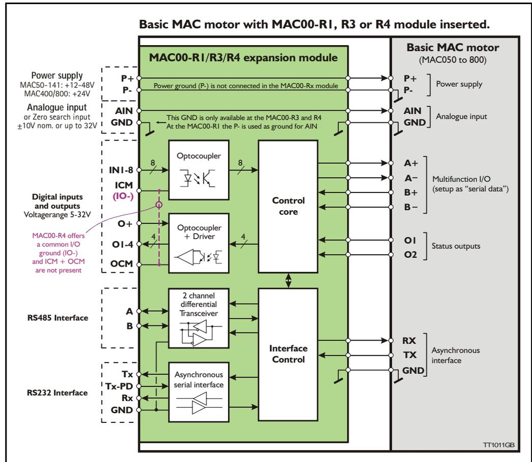
The following illustration shows how the I/O are internally connected.
