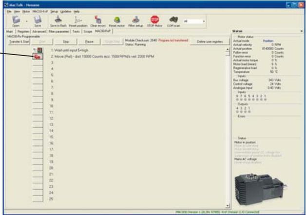
**7** The relative move command just entered is converted into a program line.
