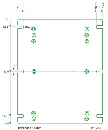
In situations where a 19" rack system cannot be used, all models using JVL's standard cabinet can be mounted on a plane surface using a Baseplate.
